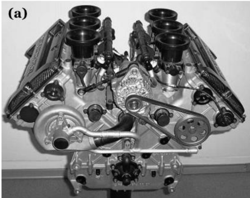
Figure : (a) V6 internal combustion engine from a Mercedes-Benz, (b) Electric motor
